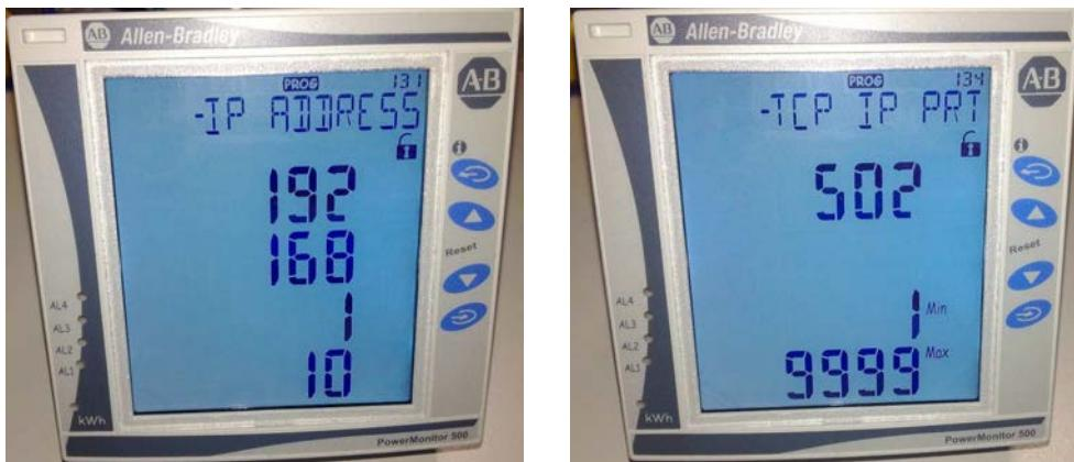
5. Connect the PowerMonitor 500 unit to the personal computer Ethernet port by using a crossover or straight-through<sup>(1)</sup> patch cable. The connection must be point-to-point without a router or any other network devices.
