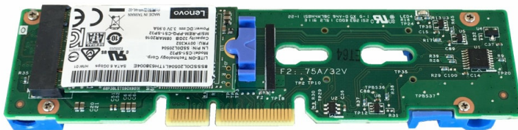
Figure 13. ThinkSystem M.2 Enablement Kit (shown with an 32 GB M.2 drive, not supported in the SE350)
