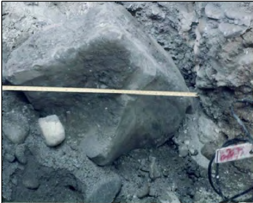
Photo No. 5. Boulders encountered at the Main Yard and Shops (currently LAUS). Photo taken: 01/18/90. Source: SCRTD, 1990b.
