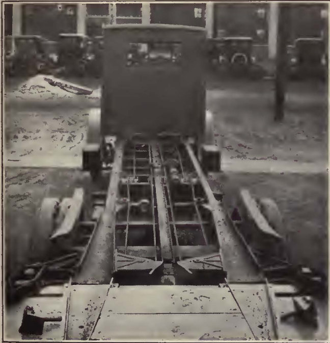
Loading Mechanism and Channel Tracks Are Bolted to Chassis. Channelways on Rear Can Be Adjusted for Height to Meet Similar Channels on Platform. Hooks Hold Front Container to Truck
