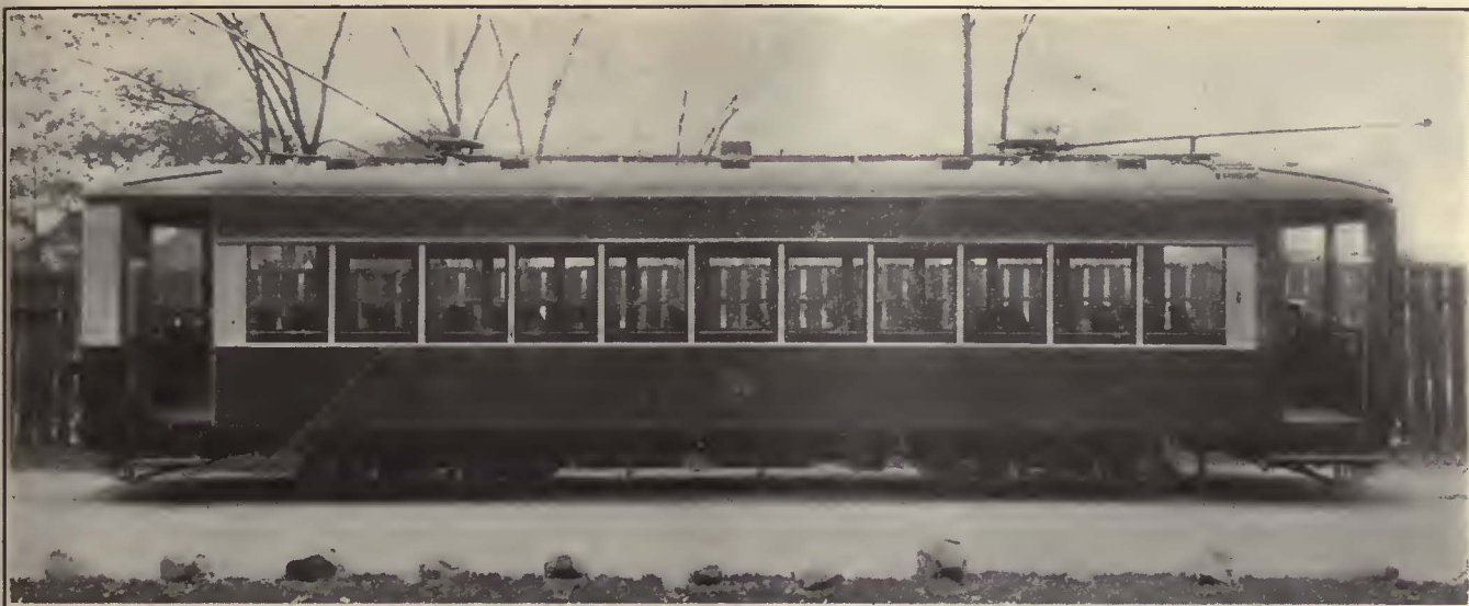
Single Sash Windows of Unusual Height Admit Plenty of Light in the New Cars of the P-O Electric Company
