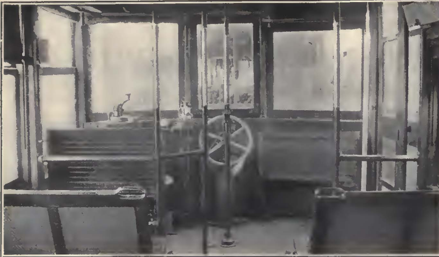
The Iron Pipe Stanchions In the Cars of the North Texas Traction Company Are Covered with Aluminum Tubing
