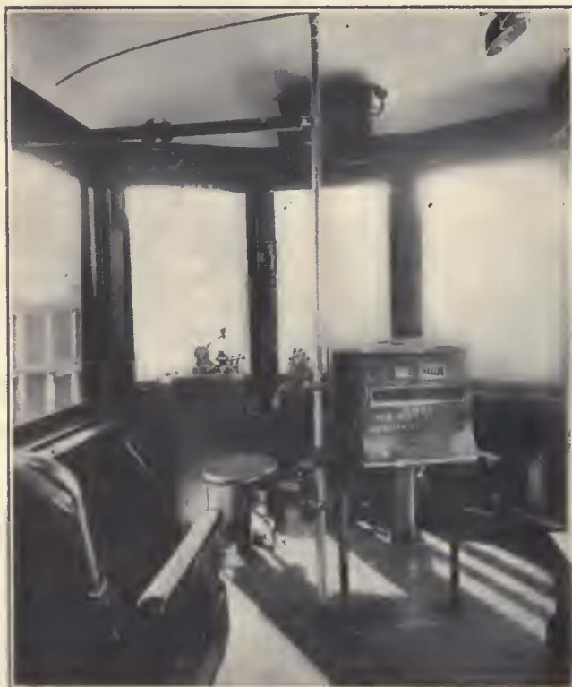
Air Pipes Leading to the Engineer's Valve Are Hidden Behind a Sheet-Iron Shield
