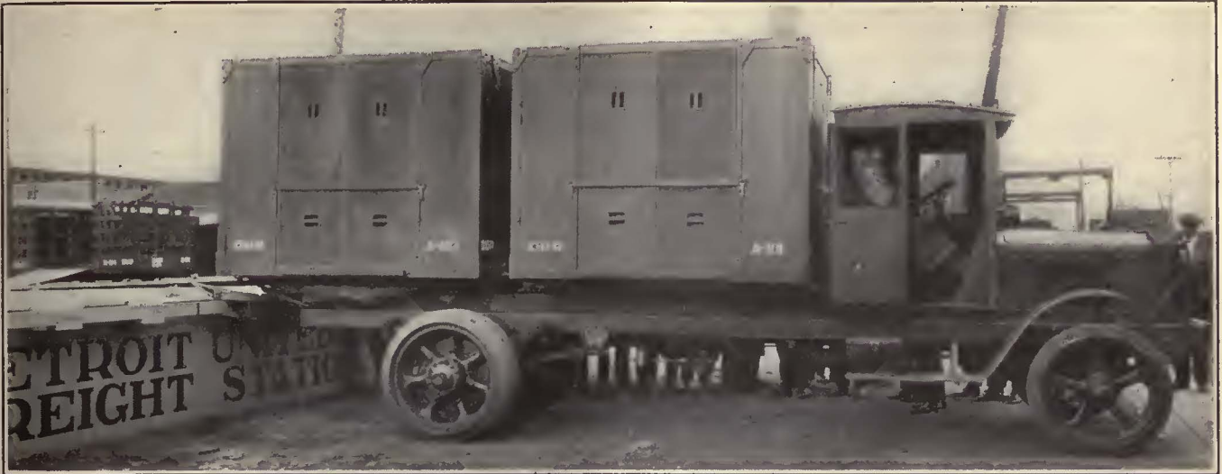
These D. U. R. Containers for Less-than-Carload Service Have 2½ Tons Capacity and Can Be Shipped Sealed from Origin to Destination
