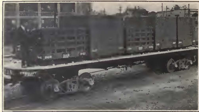
Containers When Mounted on Flat Car Are Locked in Position
