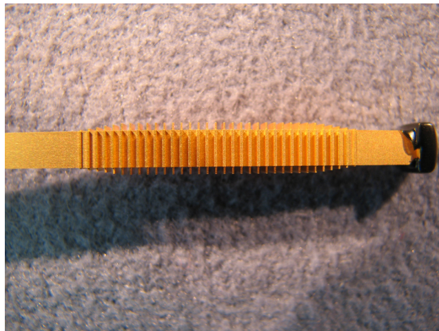
Figure F.2.5. Mandrel of the 75–110 GHz phase shifter with vane thickness 0.005 inches machined in the NTC machine shop. After electrodeposition of a thick copper layer, the mandrel will be dissolved, leaving in place its 3-dimensional negative.
