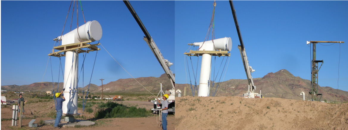
Figure F. 2.4. EVLA 2–4 GHz feed under test at the outdoor antenna test range at the AOC.
