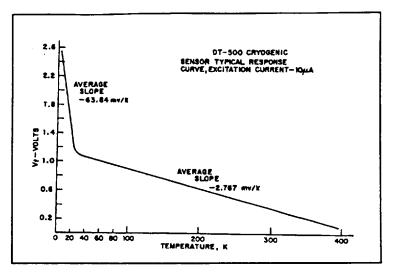
Figure 3 DT-500 Sensor Temperature Response
