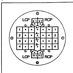
Figure 4 Dewar DC Feedthrough Label
