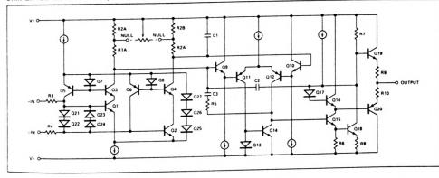
The excellent specifications of the individual amplifiers and tight matching over temperature enable construction of high-performance instrumentation amplifiers. The designer can achieve the guaranteed specifications because the common package eliminates temperature differentials which occur in designs using separately housed amplifiers.
