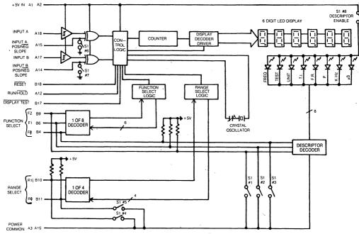
Simplified Block Diagram of a PC-6
