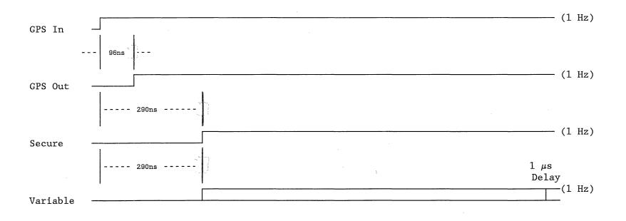
Figure 1: Waveforms of the L109
