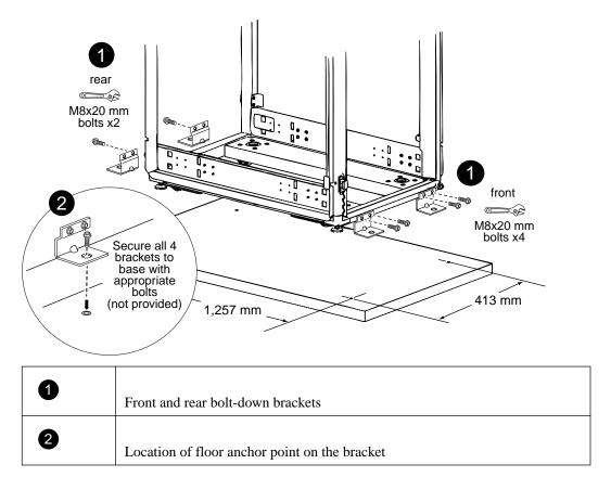
2. Mark the anchoring points where the rear bolt-down brackets will be anchored to the floor, and then drill the holes for the brackets.
