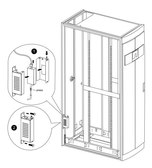
a. Lift the retaining pin on the power supply housing, and then remove the housing cover by rotating it downward and lifting it off the rear power supply housing.
