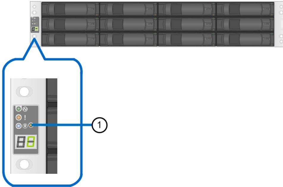
The following figure shows the ODP push button on the E2824 and E5724 controller shelf and the DE224C drive shelf.
