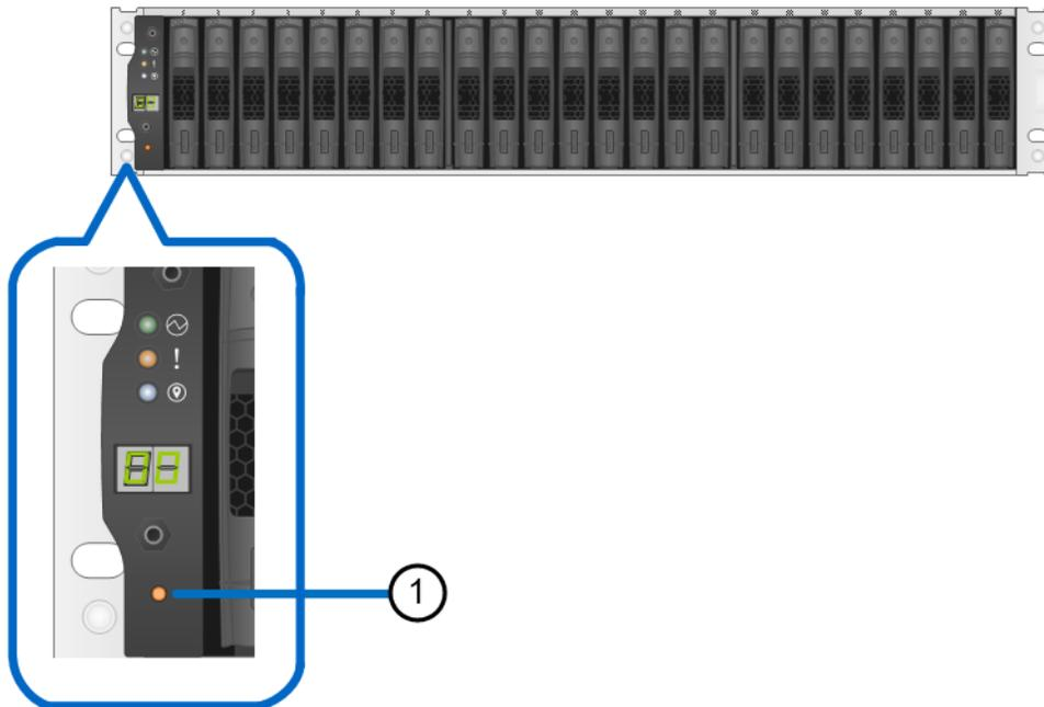
The following figure shows the ODP push button on the E2860 and E5760 controller shelf and the DE460C drive shelf.
