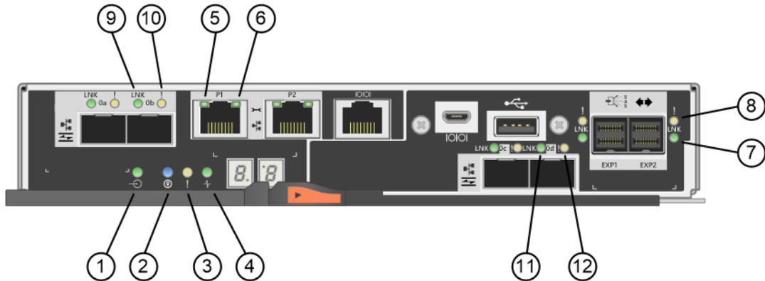
The following example shows the same LEDs on an E2800 controller with two RJ-45 baseboard host ports and two RJ-45 HIC host ports. These ports provide 10 Gbps iSCSI connections.
