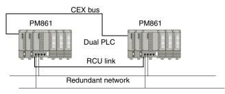
Figure 5. Example of a redundant CPU configuration.
