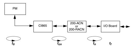
I/O Copy Time =  $t_{ti} + t_{cn} + t_{n+} t_{f}$
