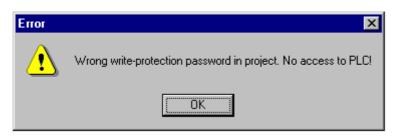
After you confirm this message with <OK>, another message appears displaying which project is loaded on the controller. Then the login is aborted.
