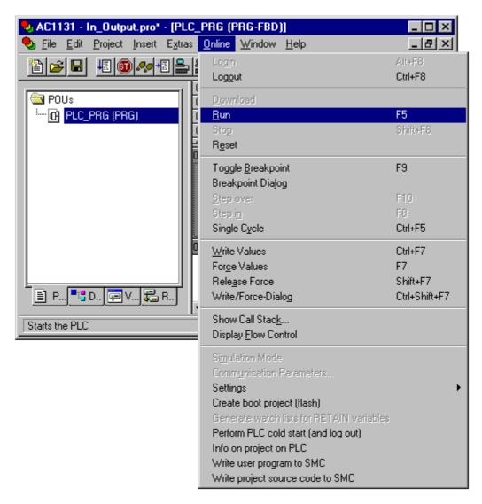
The status bar of 907 AC 1131 displays "RUN" in black color and the "RUN" LED on the PLC lights up.
