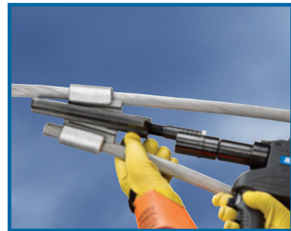
Attach power unit to tool head assembly using the unique quick-connect coupler.
