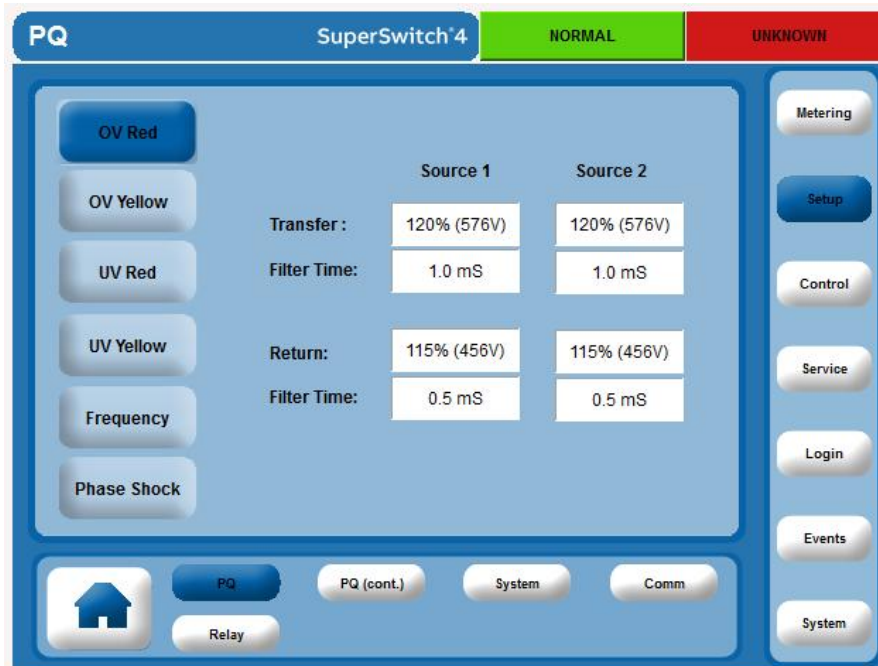
Figure 3-3 PQ Screen – Over Voltage Red
