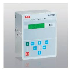
This protection device is an alternative to the similar PR521. Unlike PR521, which is self-supplied, REF 601 needs auxiliary voltage in order to function. On request, it can be equipped with all the HD4 series circuit-breakers with lateral operating mechanisms. It is the only protection device that can be installed on the HD4/R-Sec and HD4/L-Sec versions. REF 601 trips the circuit-breaker owing to:
