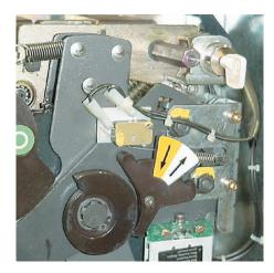
Installed in an electric circuit, this signals the state of the operating mechanism's closing springs. It is available in two alternative versions:
