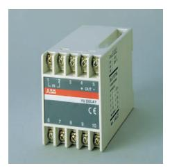
This allows circuit-breaker opening to be delayed (from 0.5 s to 3 s) when the power supply voltage drops or is cut off. It consists of a device (to be installed outside the circuit-breaker by the customer), which is interposed on the undervoltage release's power supply.
