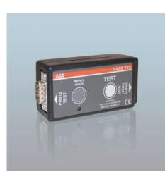
This is a portable device that allows the operation of "release chain" PR521 and the opening solenoid to be checked. It also allows the bistable alarm signalling device of the PR521 relay to be reset.
