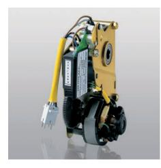
Automatically loads the closing spring of the circuit-breaker's operating mechanism. The gearmotor immediately reloads the closing spring after the circuit-breaker has closed. The closing spring can still be loaded in the manual mode (using the relative lever built into the operating mechanism) in a power failure or during maintenance work.
