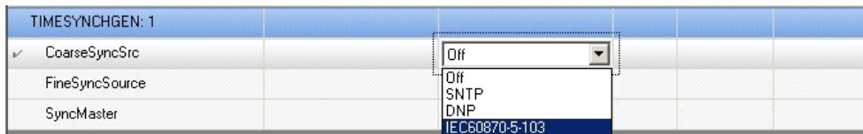
Figure 113: Settings under TIMESYNCHGEN:1 in PST
