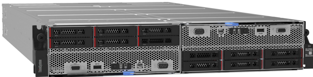
Figure 1. Two ThinkSystem SD550 V3 servers installed in a D3 Chassis
