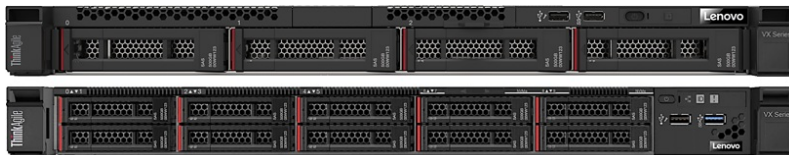
Figure 1. Lenovo ThinkAgile VX 1U Certified Node with 4x LFF (top) or 10x SFF (bottom) drive bays
