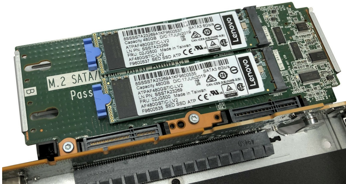
Figure 6. ThinkSystem SE350 M.2 SATA/NVMe 4-bay Data Drive Enablement Kit
