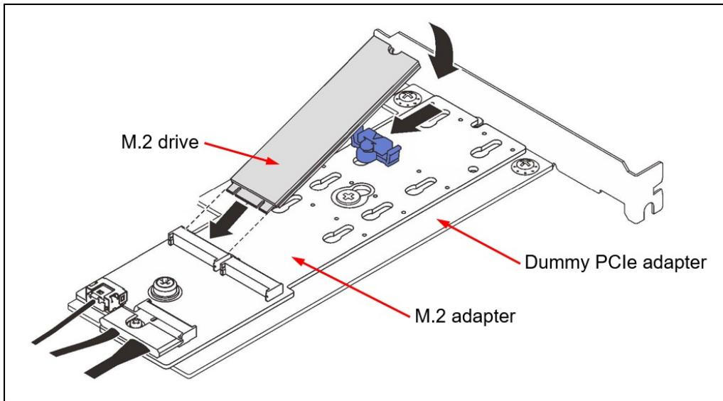
Figure 5. M.2 adapter installed in a PCIe slot
