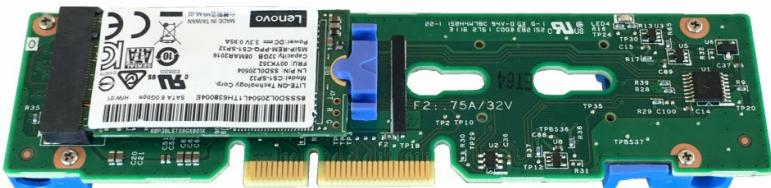
Figure 4. Single M.2 Adapter and a 32 GB M.2 drive
