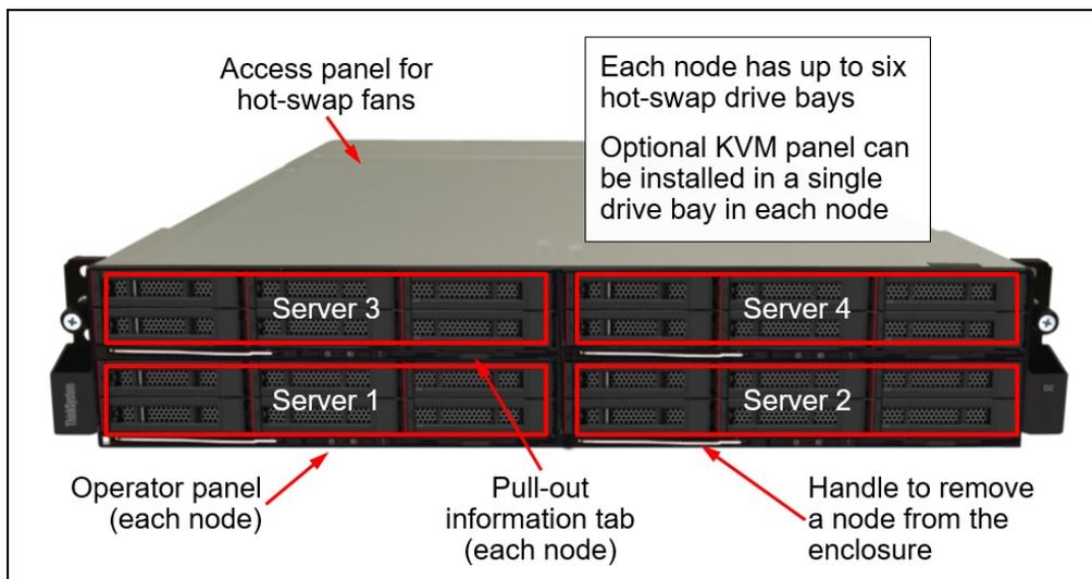
Figure 2. Front view of the ThinkSystem D2 Enclosure
