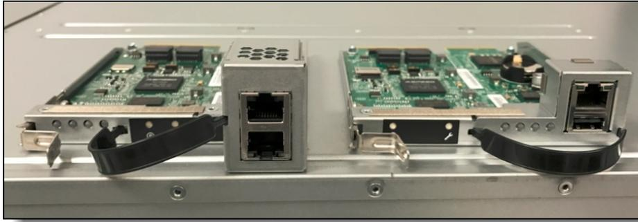
Figure 18. Dual-port SMM and standard (single-port) SMM
