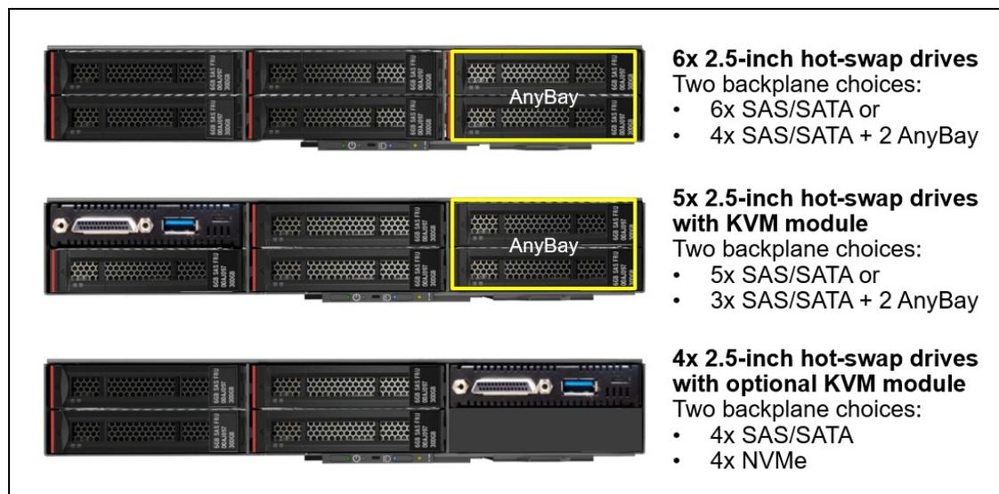
Figure 9. Drive bay configurations of the SD530
