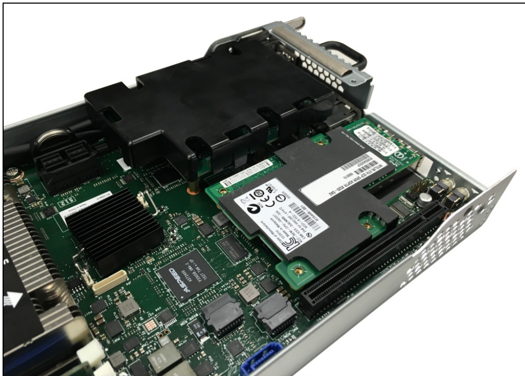
Figure 10. Adapters installed in front of the sd350
