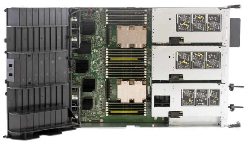
We can see the two CPUs, 20 DIMM slots (populated with 20 x 32GB DIMMs of RAM), and the two NVDIMM slots. The PCIe network AICs are also easily accessible from here.
