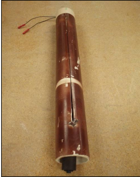
FIGURE 1. Float switch assembly installed into well screen PVC pipe
