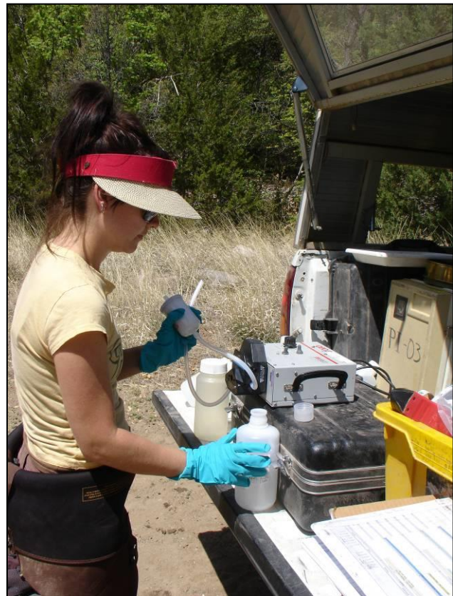
FIGURE 3.10. Filtering set-up. Note the peristaltic pump, tubing, collection bottle, receiving bottle, filter and nitrile gloves.
