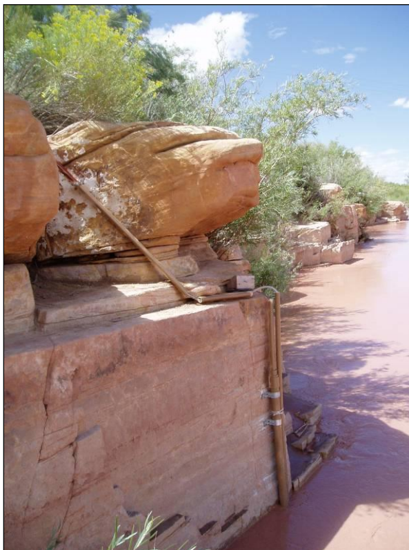
FIGURE 6.4. Examples of intake tubing (with strainer attached) and float switch installations, note anchoring to fix objects.
