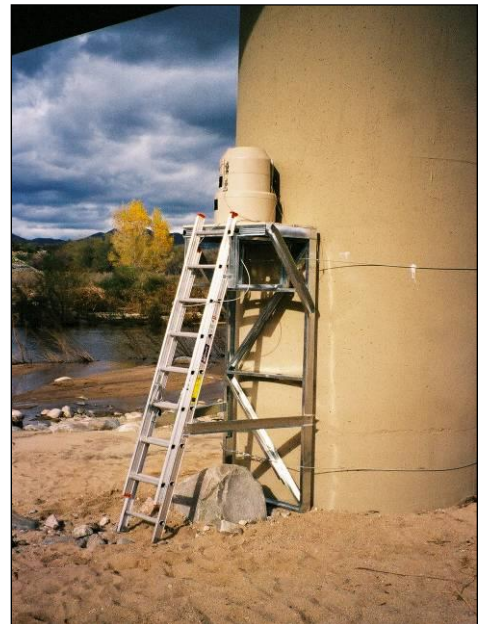
FIGURE 6.3. Example autosampler installation scenarios- under bridge (left) and secured to bridge support (right)
