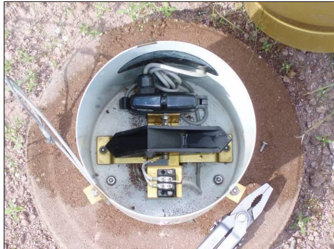
FIGURE 6.1. View of rain gage with funnel and screen removed. Note that the tipping buckets are free of any cables or wires that may hinder them from moving freely.
