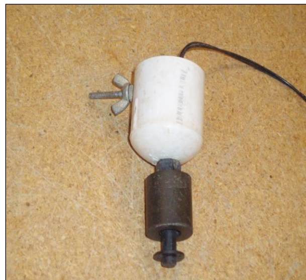
FIGURE 6.5. Float switch (black) connected to PVC cap
