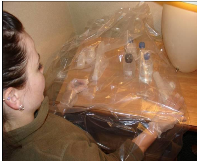
FIGURE 3.13. Field filtering of clean metals.
