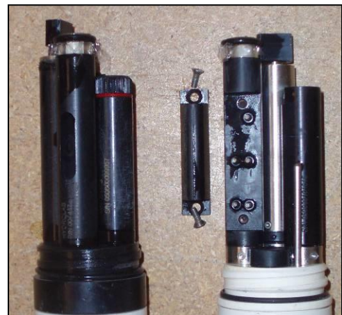
FIGURE 9.3. New graphite conductivity sensor (left). Old nickel conductivity electrodes (right). Both are combined with the DO probe.
