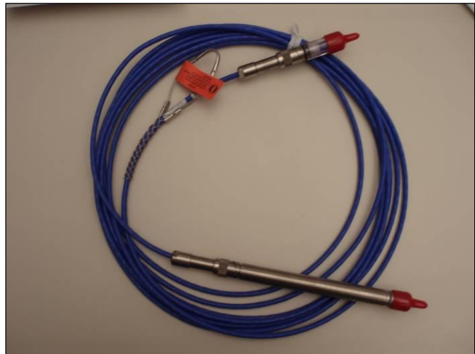
FIGURE 6.9. In-situ Water Level Logger with vented cable attached
