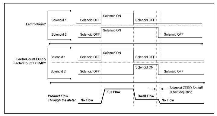
Figure 4: E-7 Valve operating sequence.
