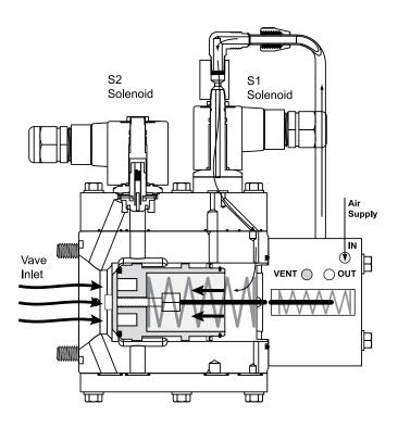
THE PORTS OF THE AIR SWITCH ARE SHOWN FACING THE FRONT FOR INSTRUCTION PURPOSES ONLY. They must be oriented so that the ports face the top or bottom of the air switch. The system is shipped with ports facing the top, which is the recommended orientation. A vertical position allows any condensation from the air pump to drain.
