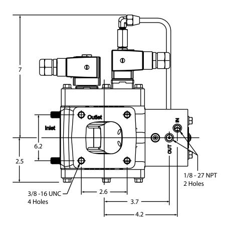
The ports of the air switch are shown facing the front for instruction purposes only. They must be oriented so that the ports face the top or bottom of the air switch. The system is shipped with ports facing the top, which is the recommended orientation. A vertical position allows any condensation from the air pump to drain.
