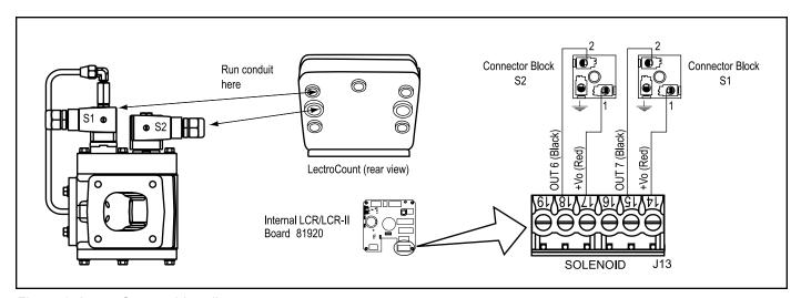
Figure 6: LectroCount wiring diagram
