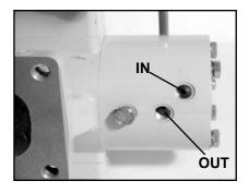
The air switch ports are shown facing the front for instruction purposes only. The recommended orientation is the top. A vertical position (top or botom) allows any condensation from the air pump to drain.
