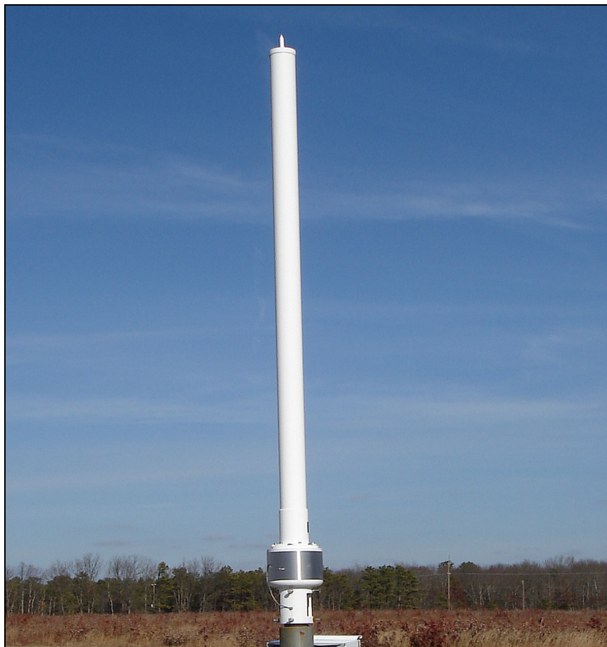
Figure 34 - The BAE GNSS Multipath Limiting Antenna (MLA)
