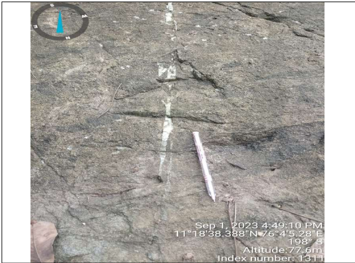
Plate 3.3 : Pegmatite intrusion along fractures in NNE – SSW direction (Source :- Photo taken during field visit by FAE) (Vintage : September, 2023)
