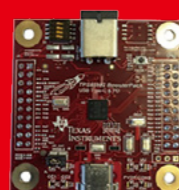
TPS65982-EVM evaluation board is a complete reference design for USB-C and power delivery
