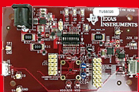
TUSB320EVM , for evaluating the TI TUSB320 USB-C port control and logic controller.
