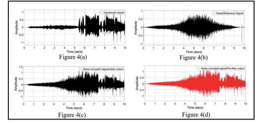
Figure 4 Input audio signal, noise / reference signal, noise corrupted signal and the pre filter output signal
