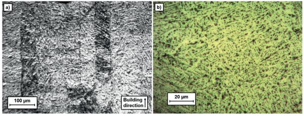
Figure 6 Microstructure of as-built Ti-6Al-4V AM sample
