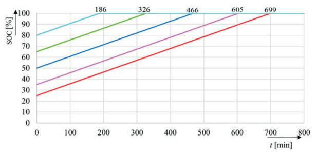
Figure 6 Charging process of EV groups within the fleet
