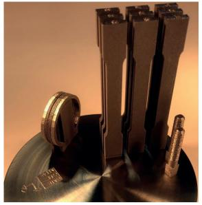
Figure 2 Tensile test sample manufacturing layout
