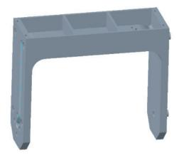
Figure 1 The original polymer bracket part
