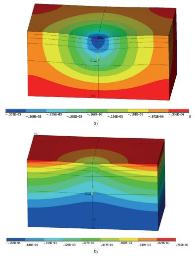
**Figure 4** Pavement deflections at temperatures:  $a \cdot T_t = 0 \circ C$ ,  $b \cdot T_t = 50 \circ C$
