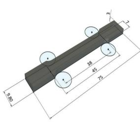
Figure 1 Tensile test sample geometry
