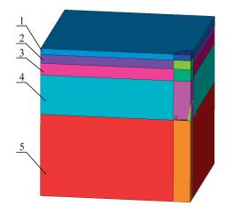
Figure 2 Structural element of the pavement. The layers of the material correspond to the pavement layers shown in Figure 1
