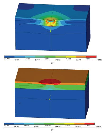
Figure 5 Distribution of the von Mises equivalent stresses in the pavement layers at temperatures:  $a \cdot T_{i} = 0$  °C,  $b \cdot T_{i} = 50$  °C
