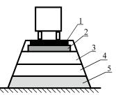
Figure 1 Estimated model of the road surface: 1 - dense asphalt concrete, 2 - porous asphalt concrete, 3 - highly porous asphalt concrete, 4 - gravel mixture, 5 - dusty sandy loam
