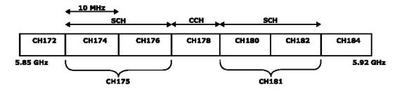
Figure 4 WAVE frequency band [26]
