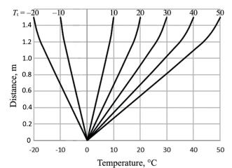
Figure 3 The obtained temperature changes in the pavement layers at different surface temperatures  $T_i$ .
