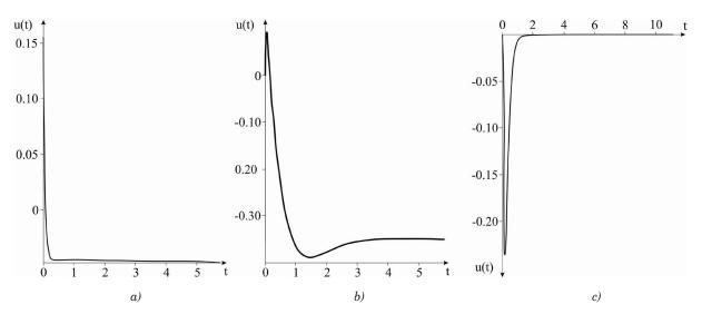
Figure 3 Variation of the lateral velocity during the transition process: a) v = 30.2 m/s, b) v = 25.61 m/s, c) v = 26.95 m/s
