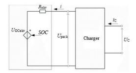
Figure 2 Equivalent circuit of a battery
