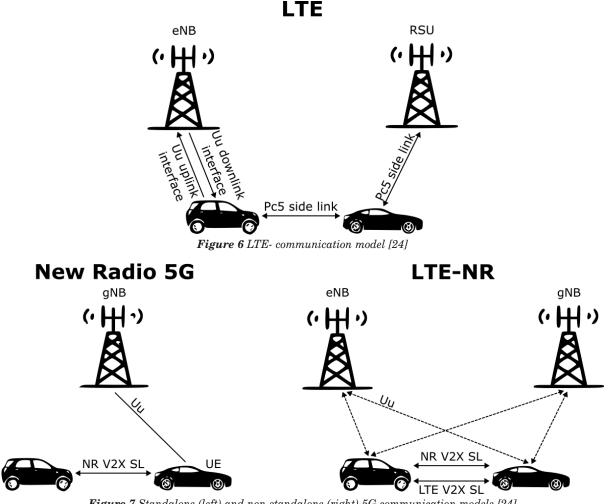
Figure 7 Standalone (left) and non-standalone (right) 5G communication models [24]
