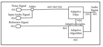
Figure 2 Active noise cancellation model without the pre-filter
