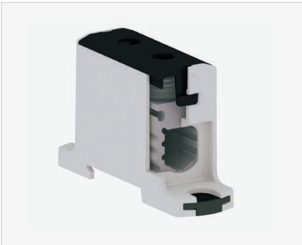
The clamp is made of a uniform flat bar covered with a special coating. Clamp screws are covered with SR1 contact paste..
