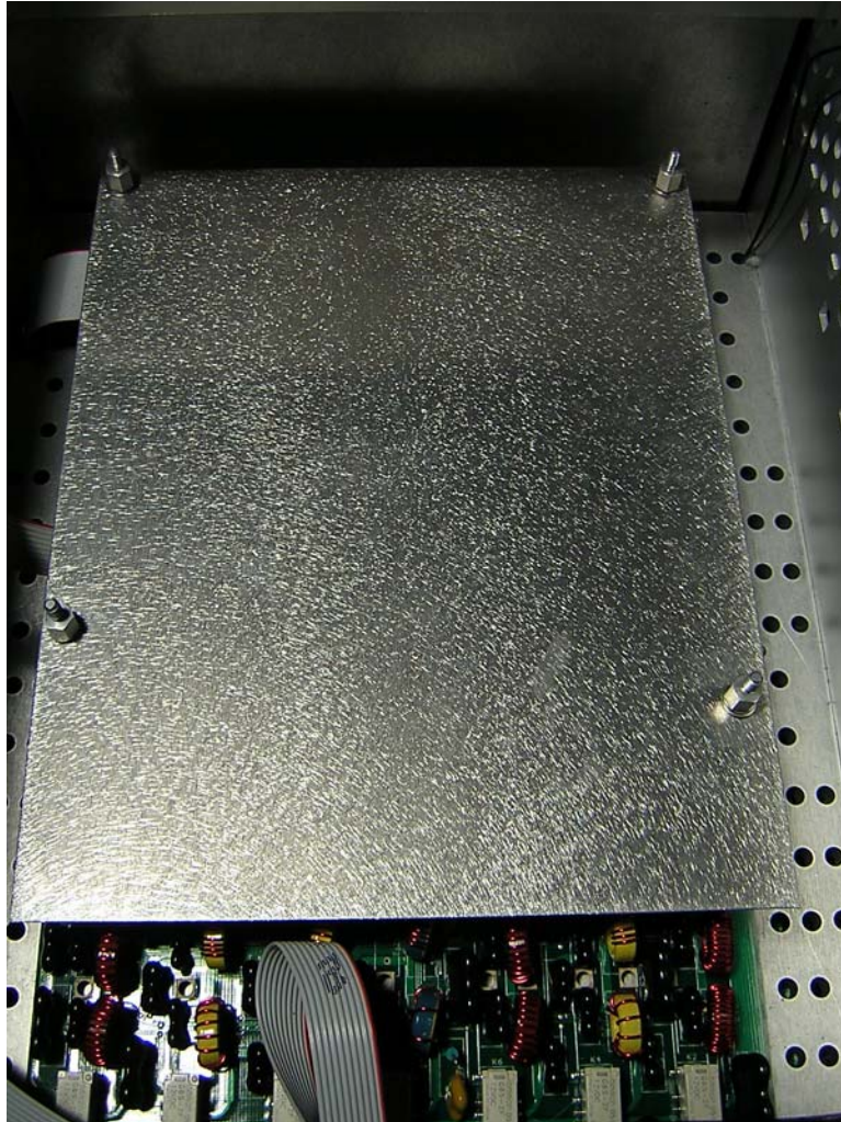
Figure 4 - Installation of four 1/4" spacers on top of shield
