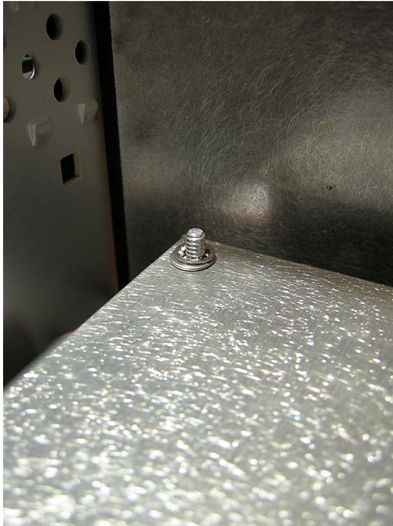
Figure 3 - Flat washer and internal tooth lock washers on top of RF shield
