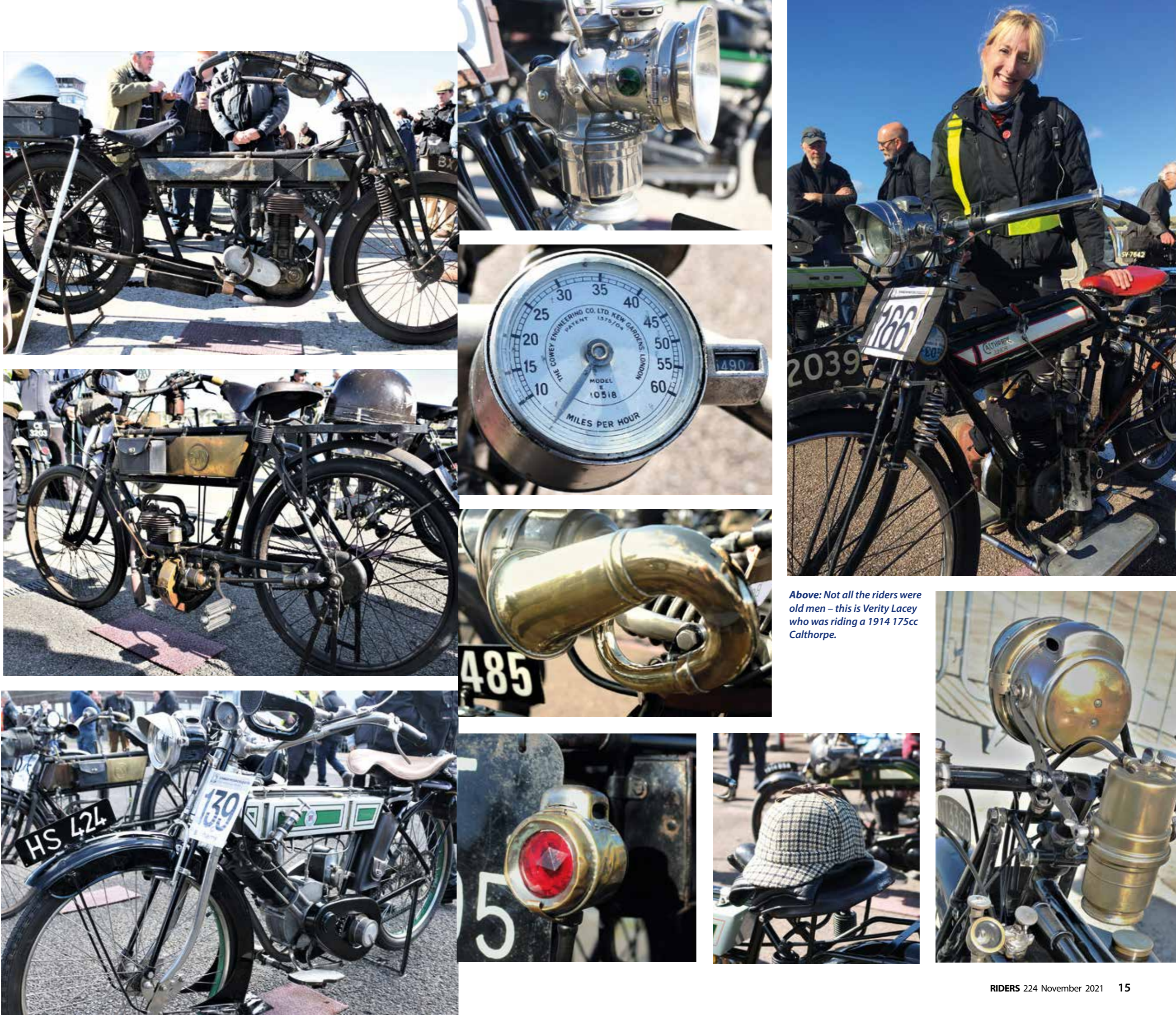
Centre: This is a 1911 247cc Belgian FN. The bike is very old but the rider was only 18. At a time when virtually everything was belt driven this bike had a posh shaft drive, yet it only had a very crude stirrup brake at the back and no front brake.
