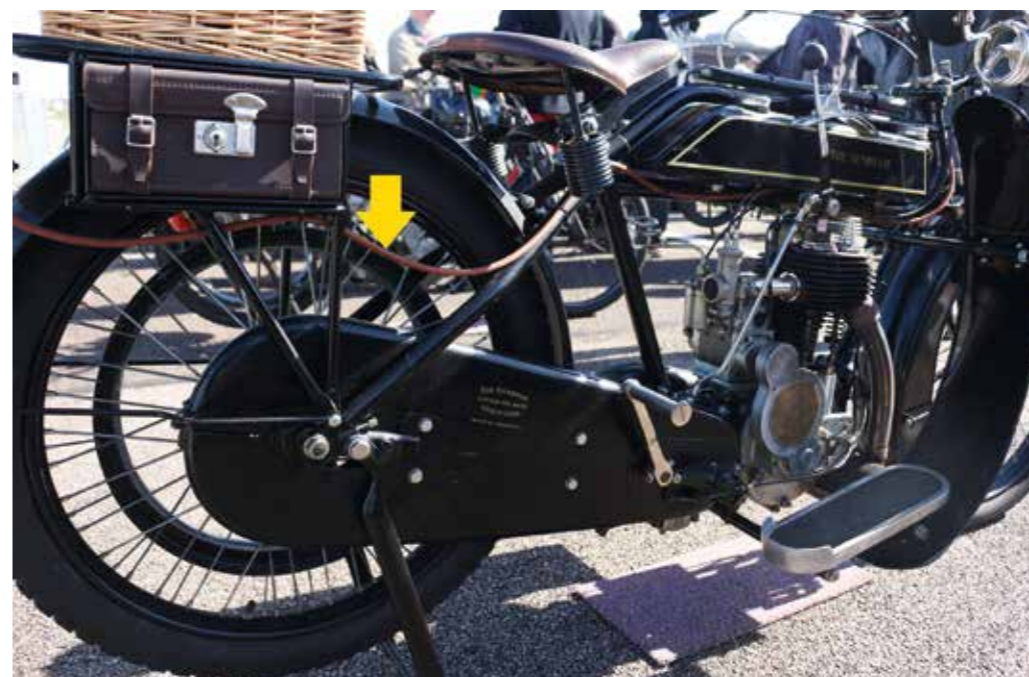
Top: A 1913 750cc 'Rudge Multi', the Bonneville of its day, with direct drive through a sort of CVT infinitely variable gear (hence 'Multi'). No rear brake and only a feeble bicycle-type stirrup front brake. Note the rubber tube taking acetylene gas to the rear light.
