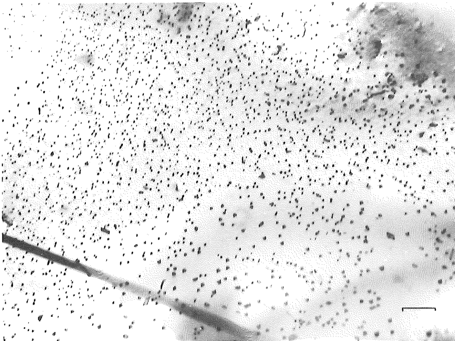
Fig.5.- a) Micrograph showing stacking-fault tetrahedra in Au+1 at.%Pt quenched from 940^\circ\text{C} to -5^\circ\text{C} and aged 1h at 100^\circ\text{C} . C_T \approx 3 \cdot 10^{15}/\text{cm}^3 . The beam direction is near to [100] and the marking indicates 2500 \text{ \AA} .
