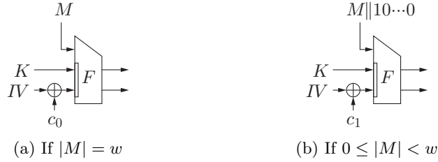
Fig. 2: The proposed hash function for at most a single-block message
