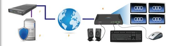
A DXT-H4 (1) connected to a closed host system (2) facilitates a remote desktop connection over a LAN/WAN (3) to a zero client (4) with quad video heads (5)
