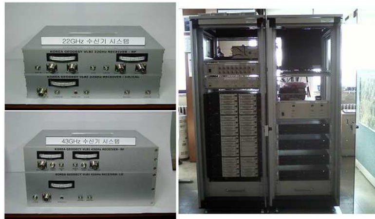
Figure 7. The 22 and 43 GHz receiver systems (left) and the K5/VSSP32 and S/X down converter (right).
