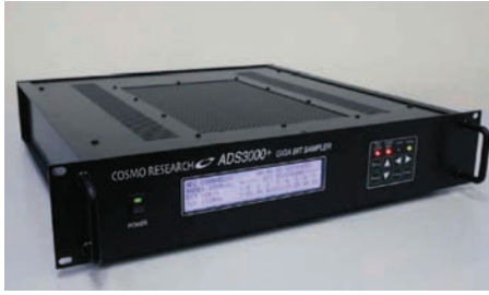
Figure 1. Front view of the ADS3000+ unit. Many status settings can be displayed and monitored.
