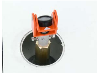
Figure 2. Retro-reflector on paraboloid surface.
