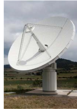
Figure 6. Patriot 12-m antenna system (photo courtesy of Jim Lovell, University of Tasmania).
