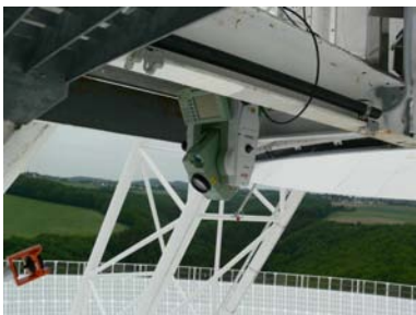
Figure 3. Leica TCRP 1201, mounted top-down.
