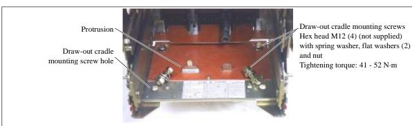
Fig. 4 Protrusion on the bottom of the draw-out cradle
