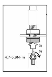
5 Wire fixing nut to a torque of 4.7 to 5.9 N.m.
