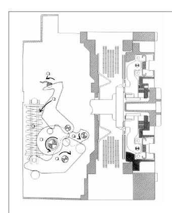
The charging handle or the charging motor provides a counterclockwise rotation to charging cam  $\ ^{\ }$  . This rotates closing release lever  $\ ^{\ }$  and closing tripper lever  $\ ^{\ }$  counterclockwise and a semicircular pawl engages with closing release lever  $\ ^{\ }$  . And charging lever  $\ ^{\ }$  rotates clockwise so that closing spring  $\ ^{\ }$  is compressed and closing cam 5 rotates counterclockwise. At this time, each component is positioned as shown in Fig. 18.
