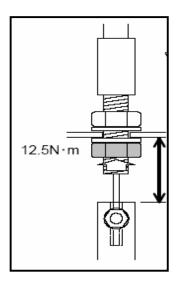
Attach the cable in the cable mounting
