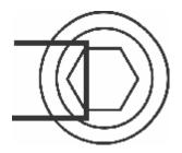
When the handle shutter is at the left of the hole, remove the adjustment plate. This will push against the handle shutter less moving it towards the centre of the hole.
