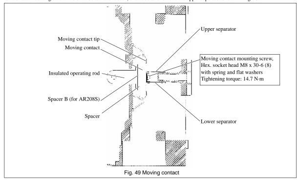
4) Supporting the spacers (the number of which varies depending on the poles), the moving contact, the lower separator, and the moving contact mounting screws by hand, turn the moving contact mounting screws additional two or three turns to remove these parts. Fig. 50 shows the moving contact-related parts.
