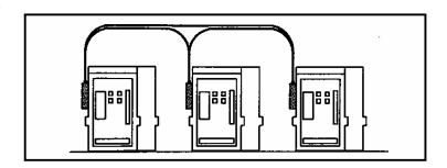
The mechanical interlock system allows up to three ACBs to be selectively turned on or off to the configured requirement.
