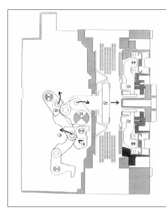
Closing cam  $^{\circ}$  rotating clockwise causes closing link and top link  $^{\circ}$  to be pushed straight. This rotates closing toggle cam  $^{\circ}$  connected with closing link  $^{\circ}$  counterclockwise, so that crossbar  $^{\circ}$  rotates clockwise and thus moving contact  $^{\circ}$  comes in contact with stationary contact  $^{\circ}$  . At this time, each component is positioned as shown in Fig. 21.
