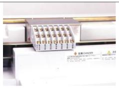
Fig. 12 Control circuit terminals
