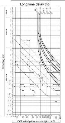
N-phase protection trip and ground fault trip
