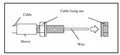
Temporarily tighten the cable 3 fixing nut.
