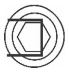
When the handle shutter is at the right of the hole, turn the adjustment plate upside down with the double side to the top. This will push against the handle shutter more moving it towards the centre of the hole.
