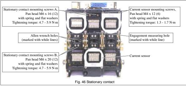
3) Unscrew stationary contact mounting screws A and B.
