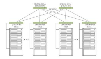
Figure 2: Edge-routed gateway at leaf with QFX5200-32C/QFX5210-64C as spine
