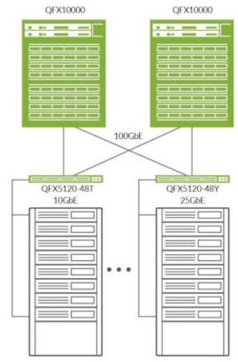
Figure 3: QFX5120-48Y and QFX5120-48T in a leaf-and-spine deployment
