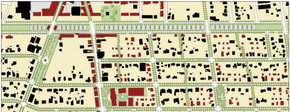
Proposed master plan showing commuter parking buffered by tree-lined thoroughfares to the north and south. Due to a lack of commuter rail service in the US, an option that removes the railroad tracks and transforms the easement to a dedicated rapid bus corridor is proposed. Given the scale of Long Beach, residents living on the edges would most likely drive from their home to the transit corridor requiring commuter parking as shown in the plan diagram above.
