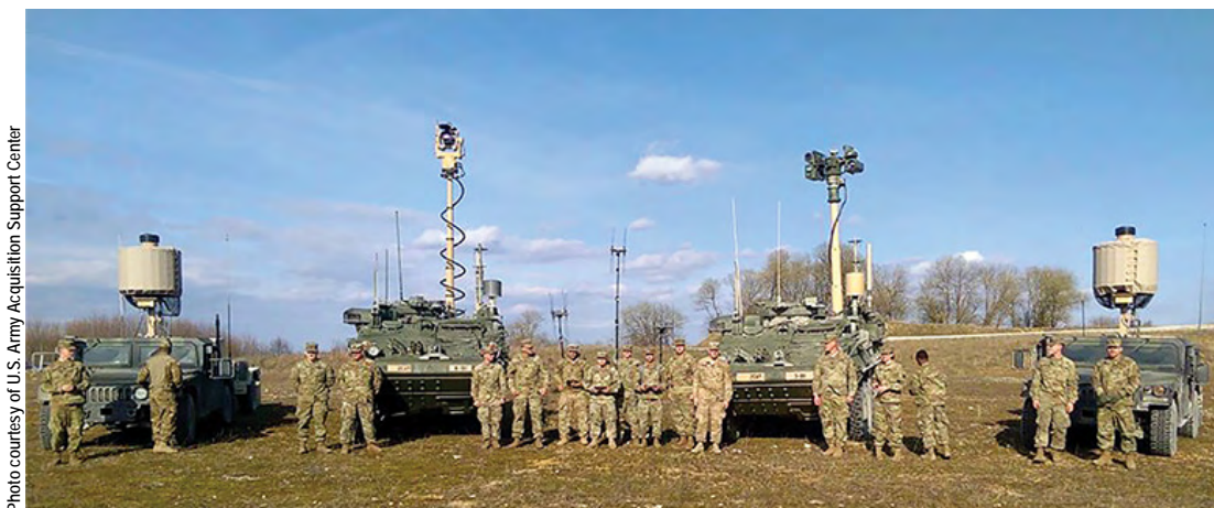
Soldiers from the 2 nd Cavalry Regiment tested several electronic warfare prototypes, including the Counter-Unmanned Aircraft System Mobile Integrated Capability, a mounted system that combines electronic warfare, radar, and optic capabilities to detect, identify, and defeat unmanned aerial threats.
