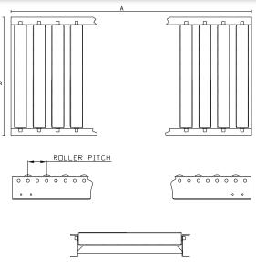
N.B. Roller sits above channel. Steel Roller 50mm Diameter Nylon Roller 48mm Diameter
