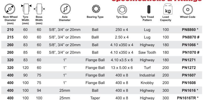
Wheel codes marked with \*Indicates 3 piece rim. All other rims are 2 piece. Recommended Max Pressure 35psi. Wheel Codes marked # are Grey Non Marking
