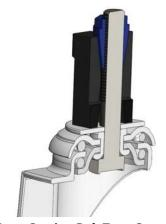
Cross Section Bolt Type Castor insterted in tube with expanding pintle part
