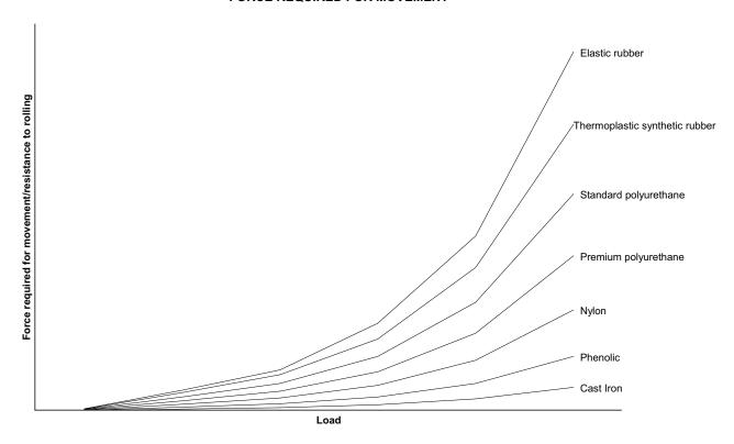
NOTE: Graph provides relative differences between wheel types assuming 150mm diameter wheels with precision ball bearings. Detailed advice can be given on request as many other factors need to be taken into account.
