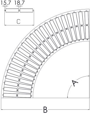
N.B. Roller sits above channel. Steel Roller 50mm Diameter. Roller Pitch is 75mm
