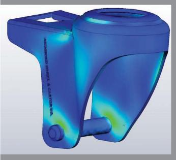
Detailed 3D stress testing using finite element analysis
