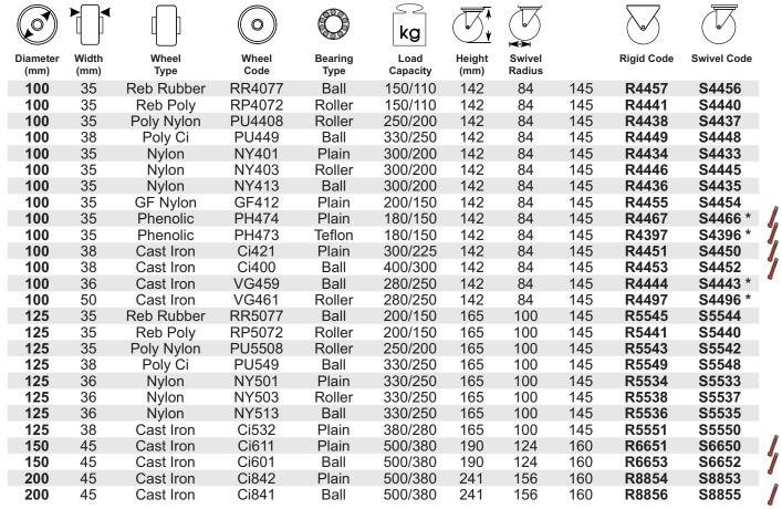
Available with a standard baseplate or M3 (Metric) baseplate. To order castor with Wheel Brake & or Directional Lock add B or D to the end of the Swivel Code e.g. S5542BD indicates a brake castor with directional lock. To order castor with Swivel Lock & Brake (SLB) add SLB to the end of the Swivel Code e.g. S4448SLB indicates a swivel lock & brake castor.
