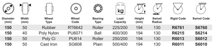
To order castor with Wheel Brake add **B** to the end of Swivel Code e.g. **S6010B** indicates a wheel brake castor. To order castor with a Swivel Lock and Brake add **SLB** to the end of the Swivel Code e.g. **S6010SLB** Indicates castors suitable for high temperature applications.
