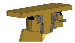
FITTED WITH LARGE DIAMETER OPPOSED TAPER ROLL BEARING SWIVEL HEAD
