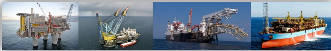
Figure 8 - From left to right: oil platform (Troll A), Lifting platform (Saipem 7000), Pipelayer (MV Solitaire), and Floating production platform (Maersk Peregrino)
