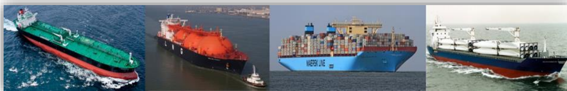
Figure 7- From left to right Oil tanker, Gas tanker (Golar Frost), Container ship (Maersk Triple E), and Bulk Carrier (Beluga Nomination)
