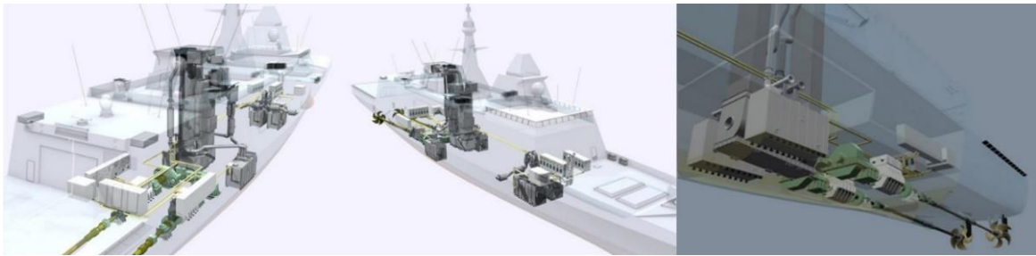
Figure 31- Arrangement of The Integrated Propulsion And Power System In The Fremms
