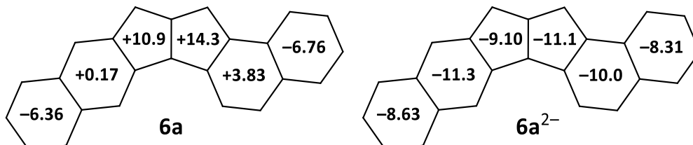
Figure S10. Summary for NICS(1) values for 6a and 6a 2- calculated at the GIAO-RB3LYP/6-311+G*/RB3LYP-D3/6-311G* level.
