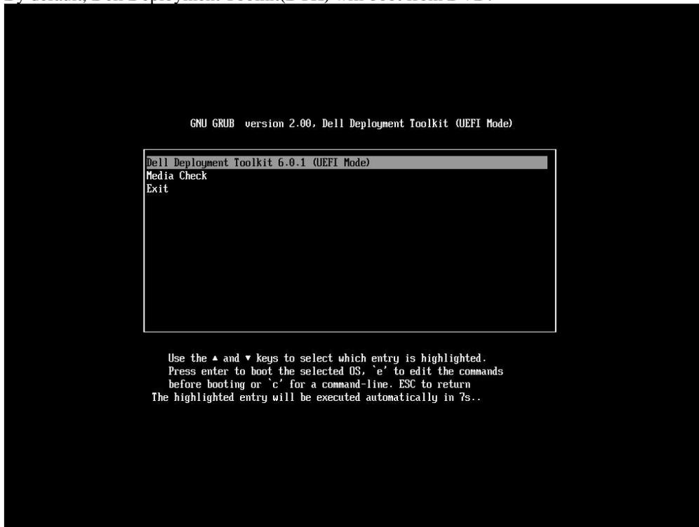
5. Booting the DTK can take up to 10 minutes. Once DTK has booted, the individual updates will begin to run. Each update determines if it is applicable to a server component and if an update of the firmware version is required. If required, an update will execute.
