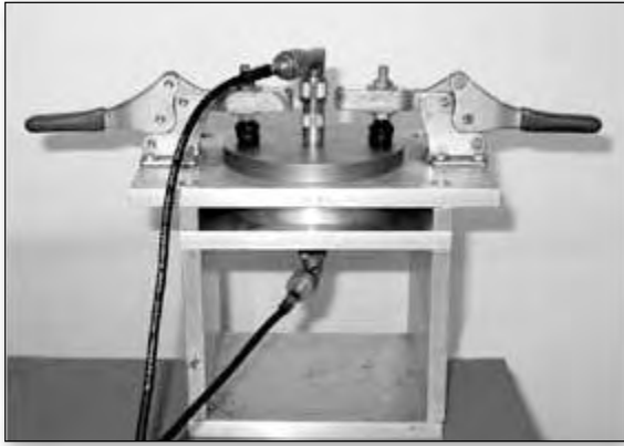
FIGURE 4: Transfer impedance – SAE ARP 1705 rev. A.
