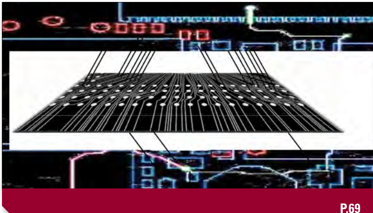
Trace clusters fanning out on a PCB: For example, in the baseband infrastructure of a handheld device. (From EMI Across Randomly-Patterned Multiple Traces on a PCB of an Audio/Multimedia Infrastructure: Crosstalk Performance Vis-A-Vis Smart Handheld Devices by Perambur S. Neelakanta & Aziz U. Noor)
