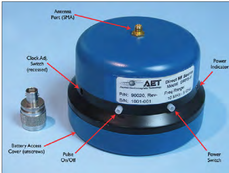
FIGURE 14: AET model DRFS comb generator. This was designed to use as a calibration source for anechoic chambers.
