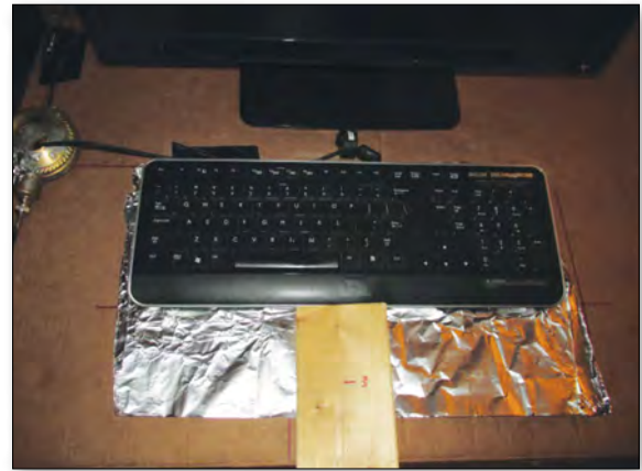
FIGURE 10: Foil placed under the keyboard—an effective solution
