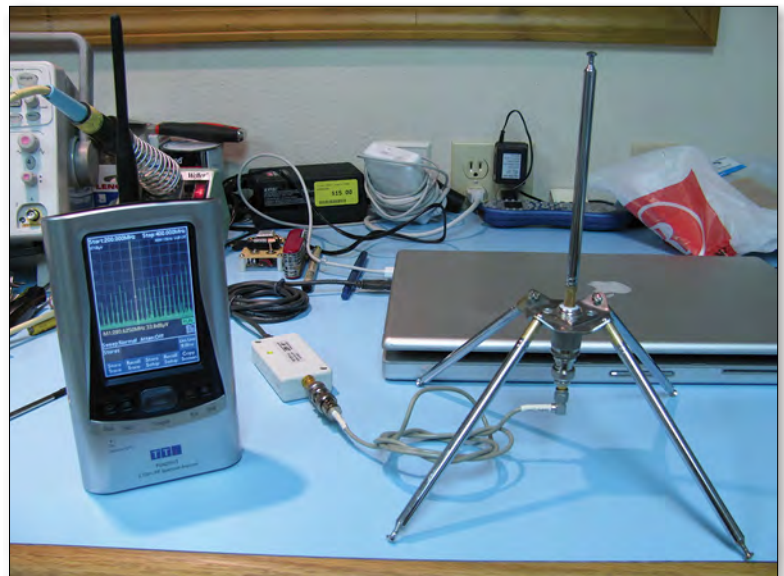
FIGURE 12: Reference antenna used for comb generator testing in a 3m chamber. The elements are telescoping, but I used it in the collapsed state to emulate a “point source” antenna.
