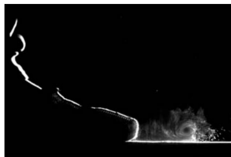
(b) Visualization of walking-induced resuspension during stomping. Reprinted with permission from [38]. Copyright 2013, Taylor & Francis.
