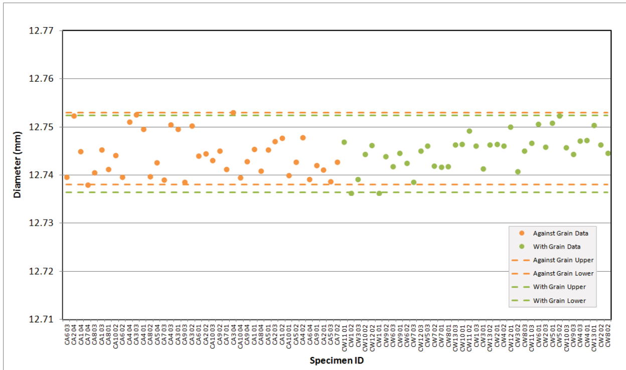
Figure A-45. H-451 Creep Pre Thermal Measurement Diameter.
