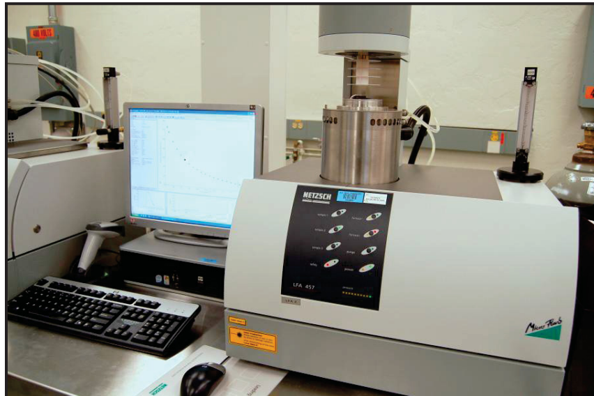
Figure 13. Laser flash apparatus measurement station for determining thermal diffusivity.
