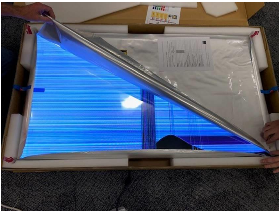
Figure 1 – Damaged UniSee panel under DOA test.
