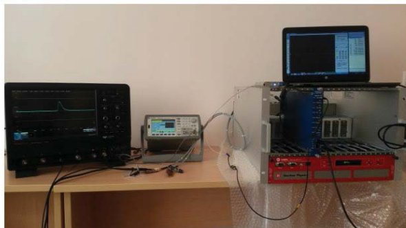
Fig.7. Test-bench for Mu2e FEE preamplifiers QA installed in DLNP, JINR.
