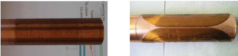
Figure 4. The thin superconducting solenoid (left side) and saddle coil (right side).
