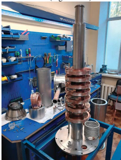
Figure 13. The gas heat exchanger
