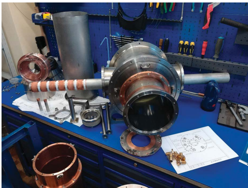
Figure 15. Pumping flanges and sintered heat exchanger
