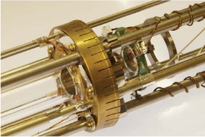
Figure 7. The SiPMs for the active polarised proton target light readout.
