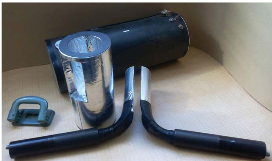
Fig.3. Detectors: E1, E2 – in the front, G1 – in the depth, scintillator with light-guide for detector M – in the middle
