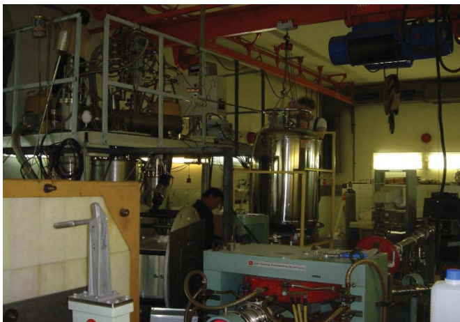
Figure 7. Target with a frozen nuclear polarization for experiments at low energies in Prague
