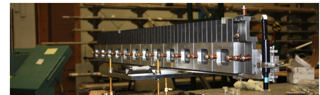
NuMI replica graphite target (120 cm, 2.5 \lambda )
