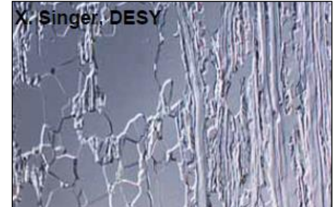
No completely recrystallized Nb
