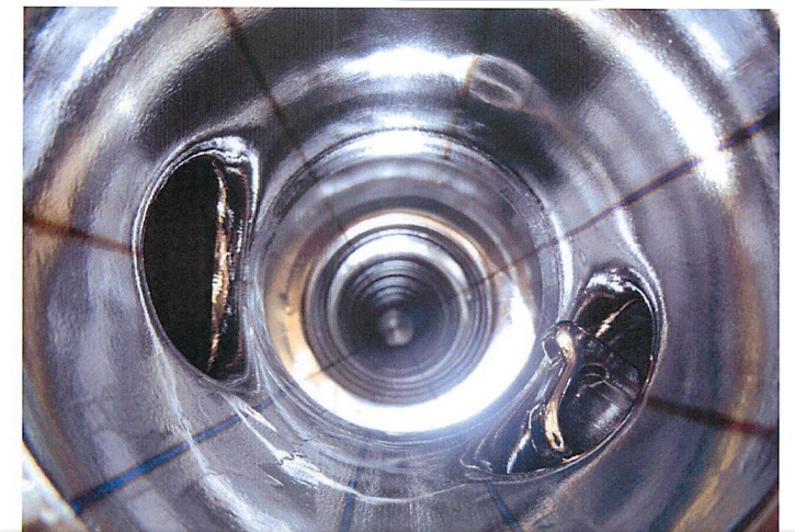
Oxidation induced by fixed HPR jets
