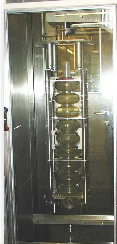
Rinsing cabinet of "new" DESY HPR system with "plastic" cavity
