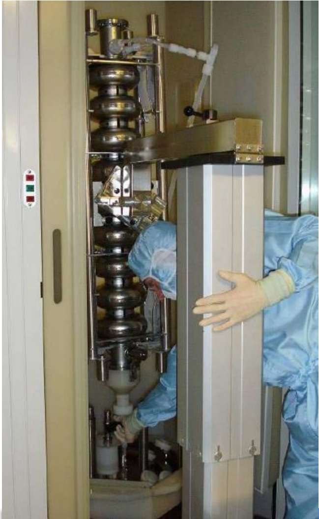
Rinsing cabinet of "old" DESY HPR system
